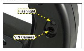
Hold Steady: Hold Controller steady when scanning the VIN barcode. This allows the user to clearly see the barcode and allows the camera to focus on it.
